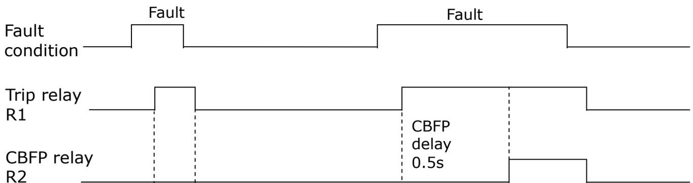
Timing diagram for CBFP. (R2 function set to CBFP, delay 0.5s.)
