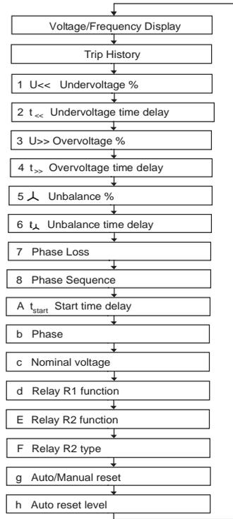
Figure 4: Display mode when pressing Reset/Mode
