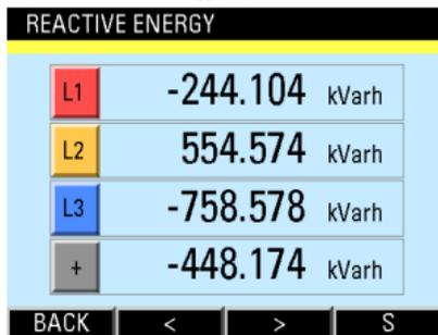
The displayed values may be incomplete due to the limited display width. Use the < and > buttons to view the complete values.
