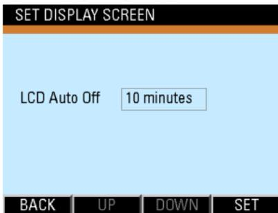
The LCD Auto Off time duration can be selected from either 5 mins, 10 mins, 20 mins, 30 mins & 60 mins or Continuous On. The default time duration is 10 minutes.
